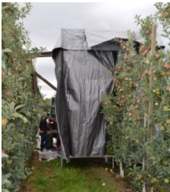
Figure 2.2: The yield estimation hardware used by Gongal et al. straddles a row of apples, blocking out light, providing a consistent backdrop and allowing imaging from both sides of the plant. (Source: Gongal et al. 2016 [28]. Used with permission.)
