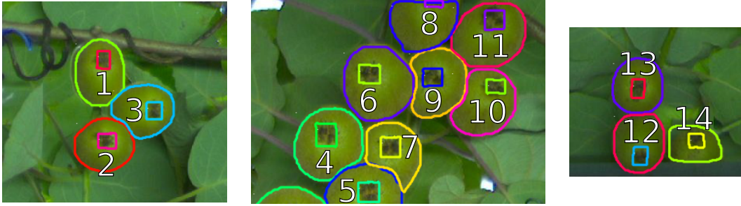
Figure 12.1: Examples of detected fruit masks. Fruit 1 and 2 have a fully convex mask outline, and are unoccluded. Fruit 3, 4, 7, 9 and 10 have partially concave mask outlines and are partially occluded. However, fruit 14 has a fully convex mask outline but is partially occluded. The calyx of fruit 1 is positioned above the centre of the fruit mask, showing that the fruit is not being viewed along its major axis. The calyx of fruit 2 is close to the centre of the fruit mask, showing that it is being view from close to its major axis.
