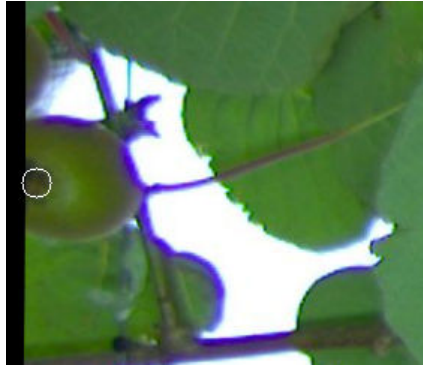
Figure 8.24: An example of a fruit detected on the edge of an image. The white circle shows the detected location of the calyx. When fruit are near the image edge, the centre of the calyx tends to be inaccurately located, which results in localisation error when stereo triangulated. The localisation error causes errors in the fruit tracking system leading double counting of fruit. Hence, fruit detected within 20 pixels of image edges are disregarded.
