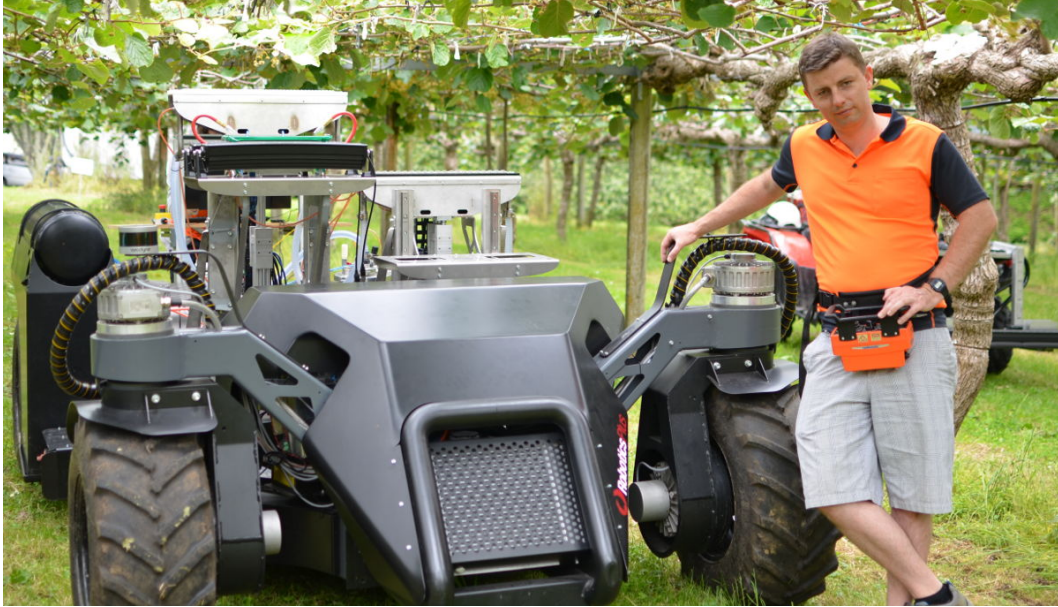
Figure 2.4: The autonomous, multi-purpose, mobile platform presented by Jones et al. [75]. The AMMP is shown with pollination equipment mounted.
