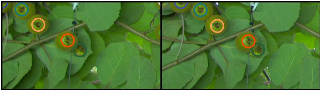
Figure 7.6: Example of a false positive match. The match marked in green is not a fruit, but a dead leaf. The detection system has misclassified the leaf as a calyx in both images and the matching algorithm has matched it.
