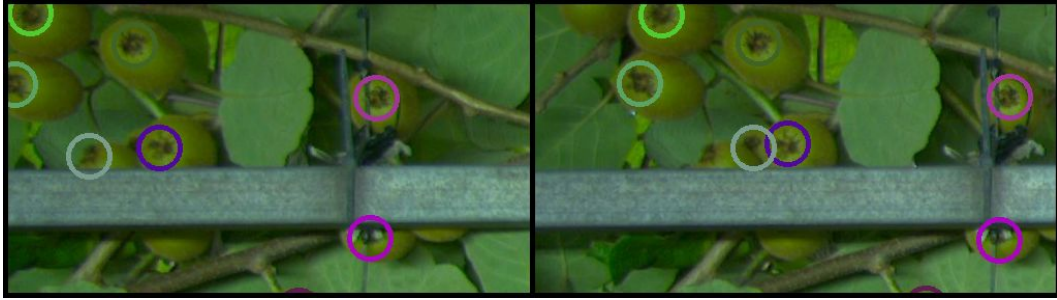
Figure 7.7: Example of an incorrectly matched fruit. The match marked in grey is not the same fruit in both images. There are three fruit in a cluster with the middle fruit being partially occluded by the other two. All three of the fruit are detected in the right image, but the middle fruit is not detected in the left image. The missed fruit resulted in an incorrect match being found.
